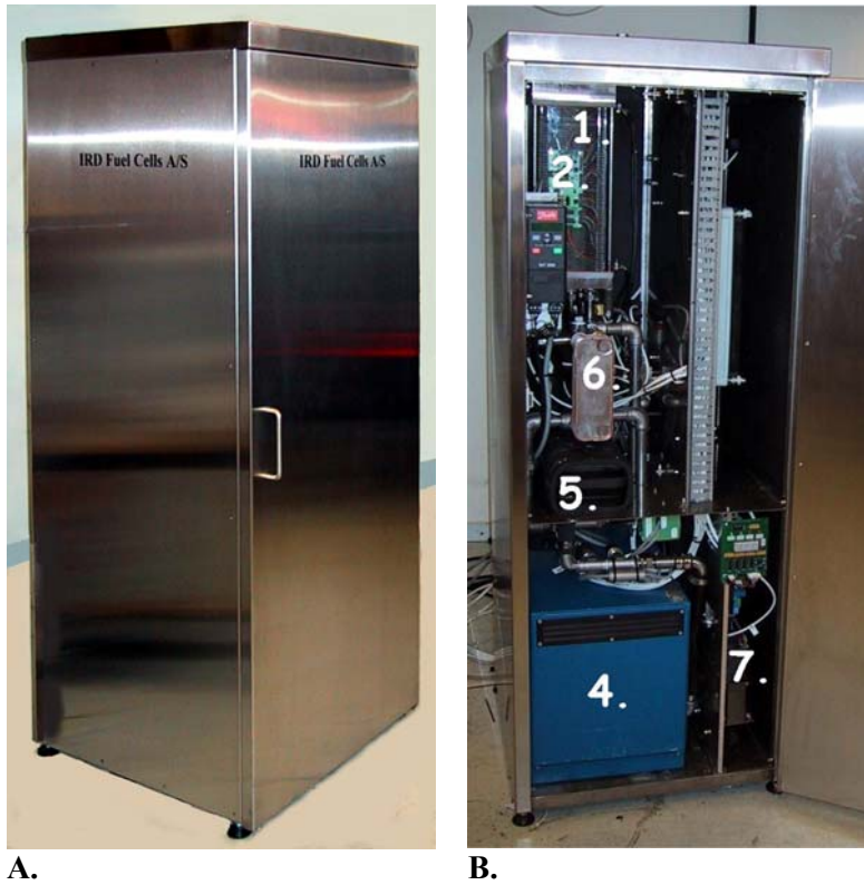
Figure 3. IRD's prototype micro-CHP.
