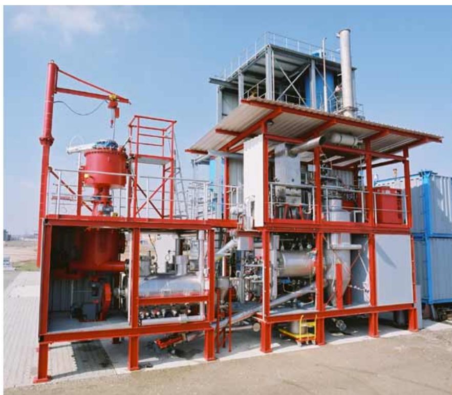
Figure 9. Small scale Gasifier Carbo compact, 150 kW e , Picture courtesy of Technischer Apparatebau Freiberg
