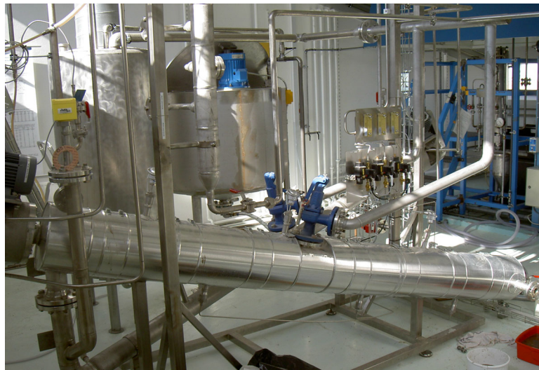
Figure 2. Risø's pilot plant reactor (1-10 kg/hour) for pre-treatment of biomass for ethanol production
