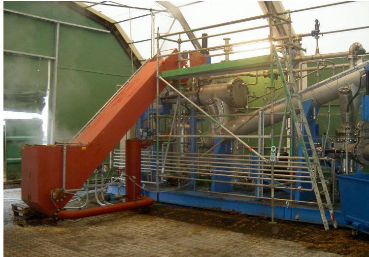
Figure 1. Pilot plant reactor (100 kg/hour) for pre-treatment of biomass for ethanol production placed at Fynsværket in Odense
