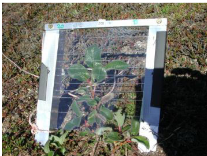
Figure 1. A Salix arctica shoot fixed with nylon strings in an elevated position. A transparent Mylar ® filter is placed above the shoot
