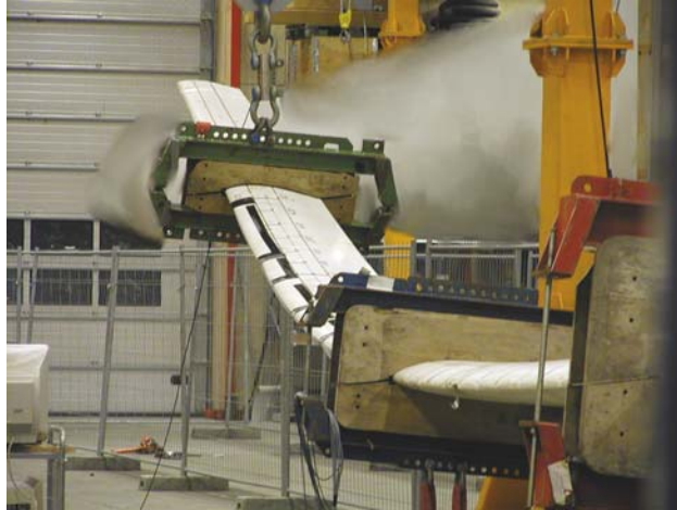
Fig. 2.5 Test of section 1; the blade deflects significantly before failure occurs.
