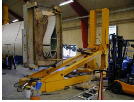
Figure 10 Test of section 3 with load introduction at 11.3m Figure 11 Failure 4.4m from the root.
