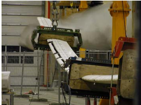
Figure 7 Test of section 1, large deflection is seen in this test.
