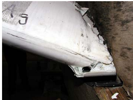
Figure 9 In test of section 2 the blade unfortunately failed at the loading yoke at 15.3m from root section
