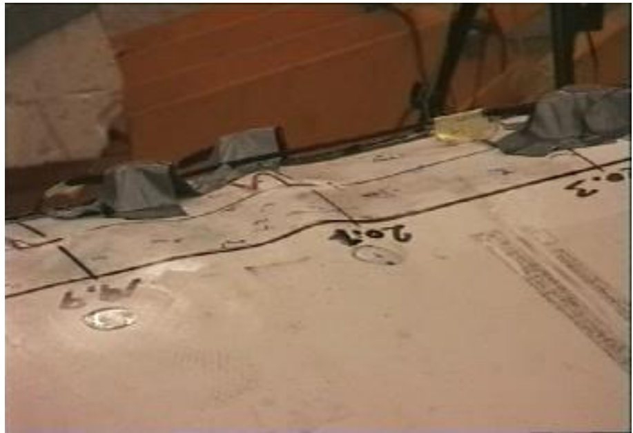
Figure 27 Photo of skin behavior (skin laminate debond from the main spar)
