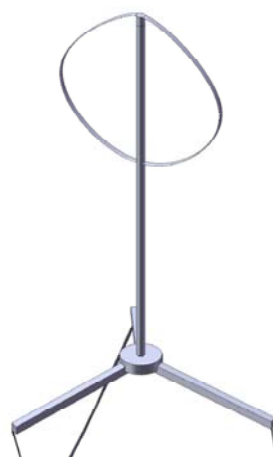
Figure 91 Darrieus rotor, torque arms and mooring system, top-view.
