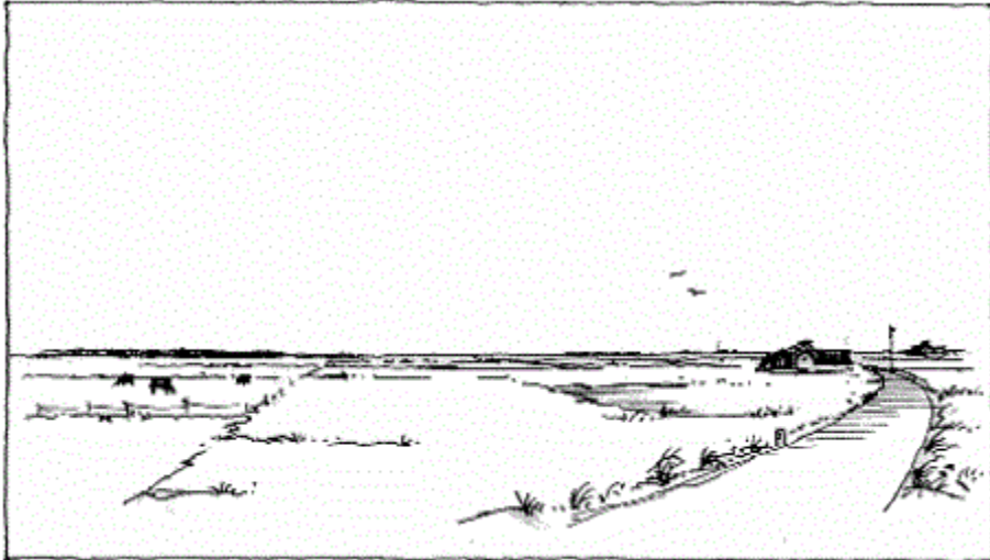
Example of terrain corresponding to roughness class 1: open areas with few windbreaks. The terrain appears to be very open and is flat or gently undulating. Single farms and stands of trees and bushes can be found. The roughness length is z_0 = 0.03 m.
