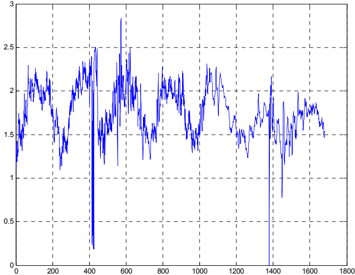
Figure 3.26. Madumvej. Week 01 + 02. Clock function in MW with 1680 parameters. A = -0.0634 \text{ MW/}^\circ\text{C} .
