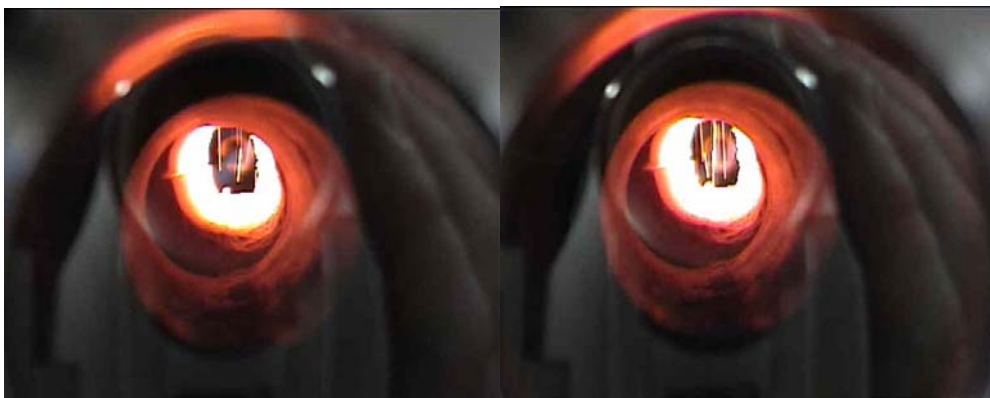
Figure 4. Burning bark particles after around 325 ms observed in position TI8. Light tracks from burning particles are at this position straight lines. No flame or soot around particles.
