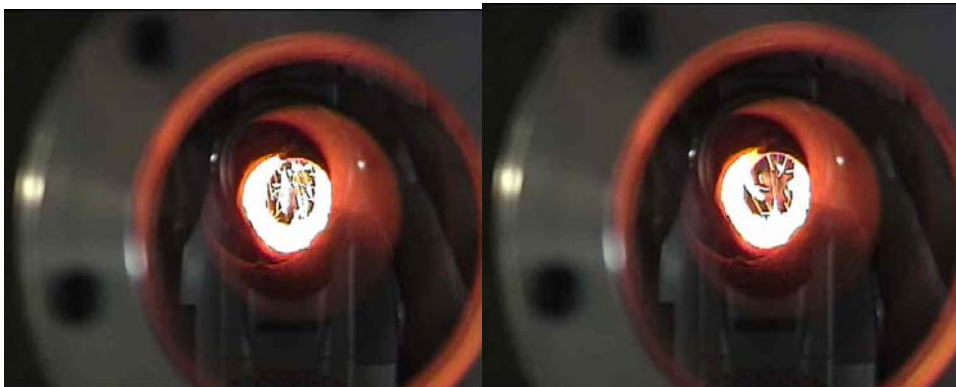
Figure 3. Ignition of bark particles after around 100 ms observed in position TI6 (flames/soot). Right a picture with a few particles and left a picture with several particles is shown. Light tracks reflect complex flow patterns of particles. Some particles are surrounded by a flame/soot .
