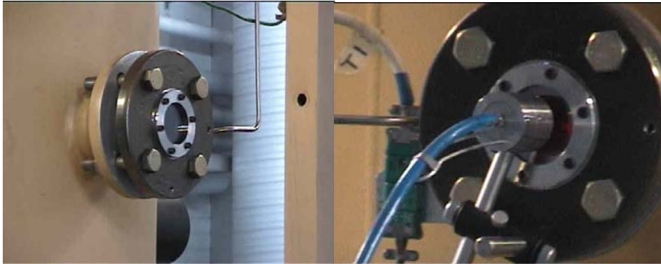
Figure 2 Left is shown a sapphire window mounted in a window section of the VTT-PEFR. Right the aligned optical sensor is mounted with a mid IR fiber that is connected to the FTIR spectrometer is shown.
