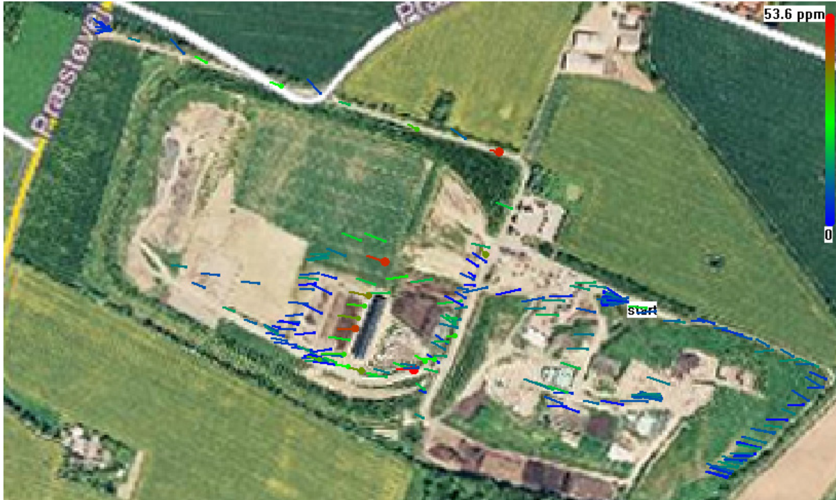
Figure 13. CO 2 concentrations at the composting facility. Scale from the 0 to 54 ppm above ambient concentrations.
