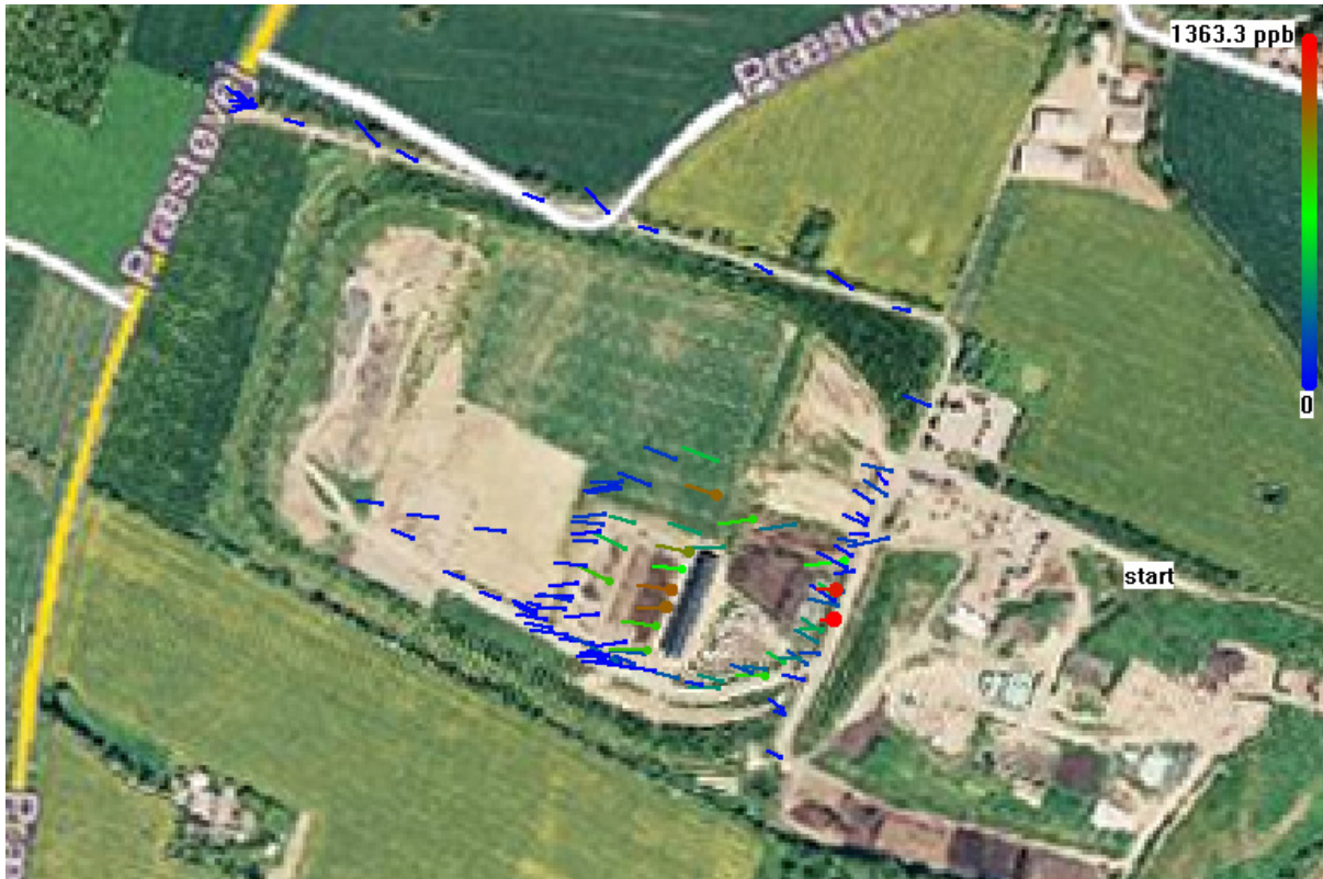
Figure 12. CH 4 concentrations at the composting facility - scale from 0 to 1363 ppb above ambient concentrations.
