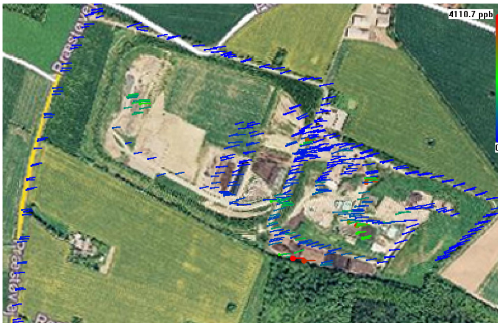
Figure 3. CH 4 leak survey with FTIR across the Fakse landfill and composting area on the 12 th of October 2006. Color scale and dot size indicate concentration of methane in ppb, sampled 2 m above ground. The scale is linear from 0 to 4111 ppb. The colored lines are pointing up in the wind, and thus indicate potential leak source area.
