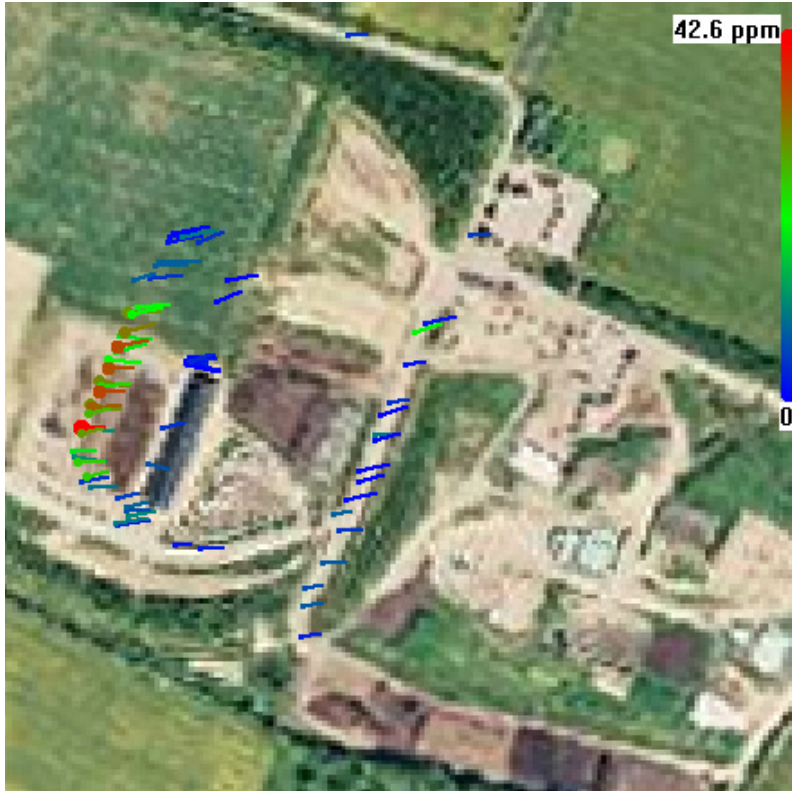
Figure 7. Concentrations of CO 2 at 2 m above ground around the compost area at Fakse landfill 061012. Color scale from 0 to 43 ppm CO 2 above ambient level.
