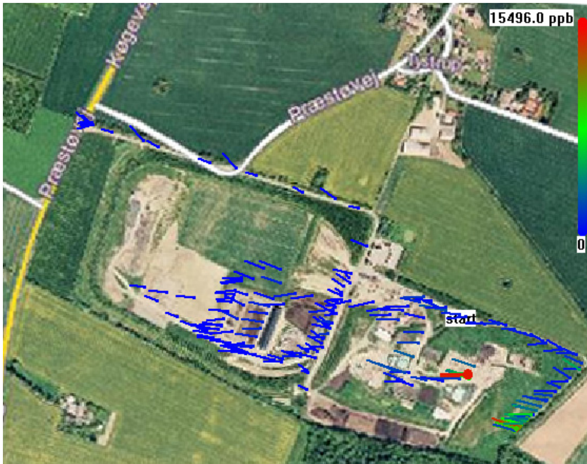
Figure 9. CH 4 leak survey with FTIR across the Fakse landfill and composting area on the 20 th of February 2007. Color scale and dot size indicate concentration of methane in ppb, sampled 2 m above ground. The scale is linear from 0 to 15500 ppb. The colored lines are pointing up in the wind, and thus indicate potential leak source area.
