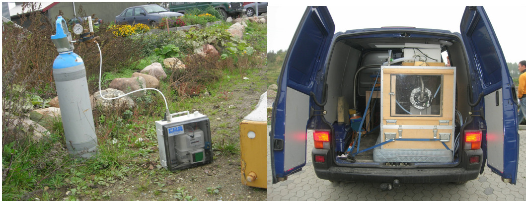
Figure 1. A: \text{N}_2\text{O} tracer release unit, including gas bottle, two-stage regulator, and volume integrator. B: The mobile FTIR instrumentation.
