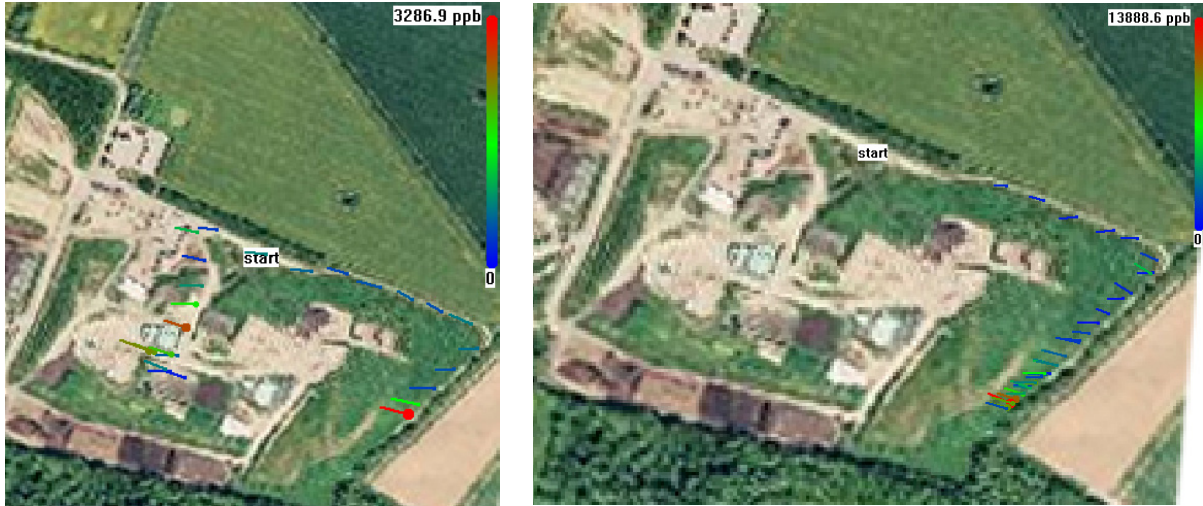
Figure 10. A: Methane concentration 2 m above ground for the central part of the landfill, with the scale going from 0-3290 ppb. B: Methane concentration 2 m above ground for the northeast corner and fence-line, but with the scale now from 0-13890 ppb.
