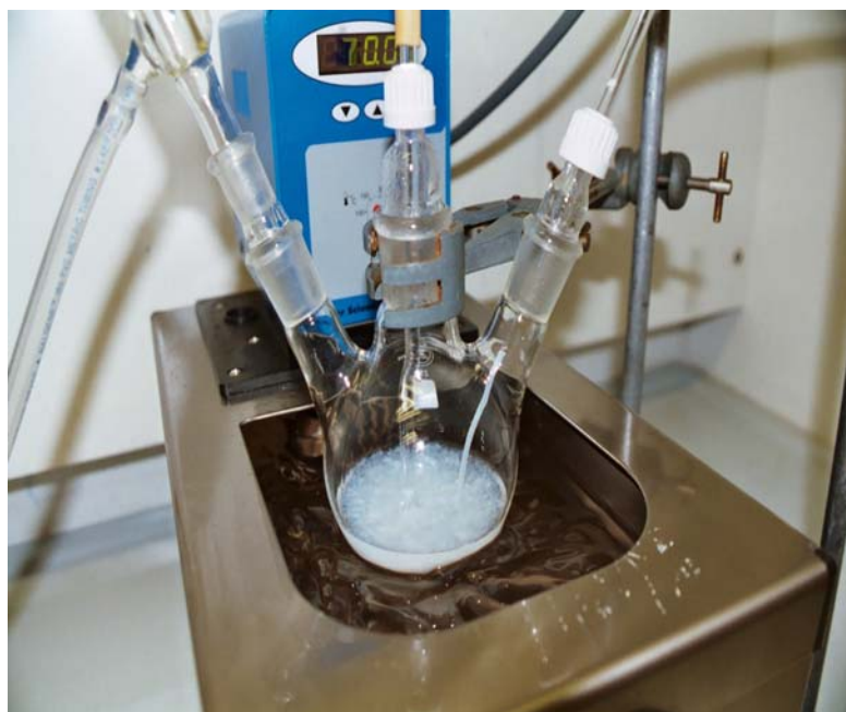
Figure 6.3 – Apparatus used for the preparation of molecularly imprinted polymers.
