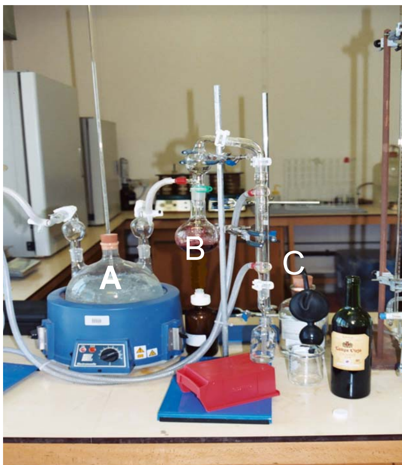
Figure 7.13 - Steam distillation apparatus. Featuring steam generating flask (A) sample reservoir (B) condenser and sample trap (C)
