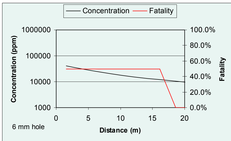
Figure 10 Concentration and probability of fatality due to flash fire in the propane jet due to liquid release through the 6 mm tubing at 2 m/s wind speed.
