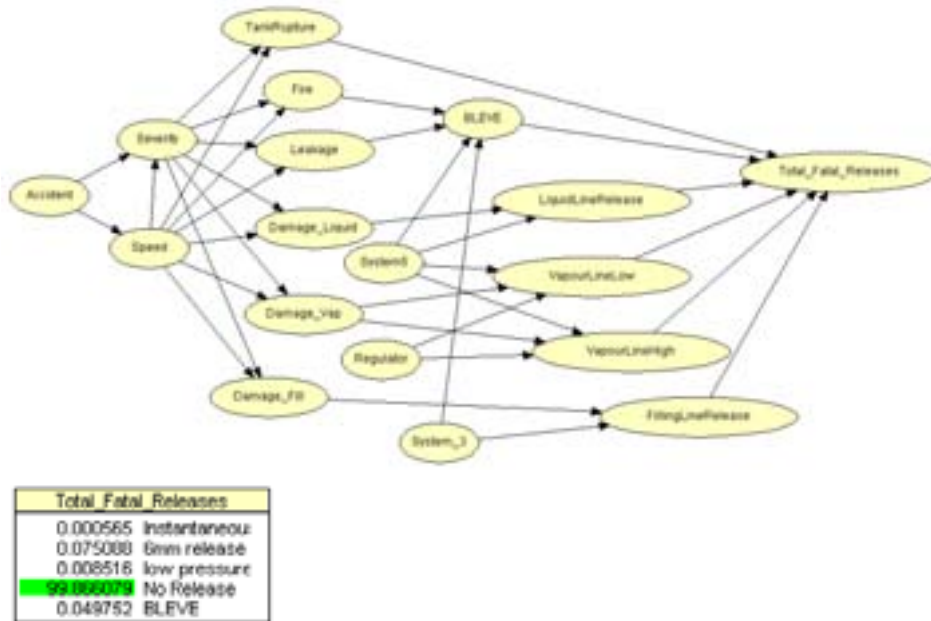
Figure 6. Bayesian belief network to analyse the likelihood of serious LPG releases with possible fatal consequences. The probability is conditional on an accident happening.
