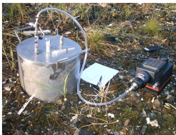
Figure 5.1 Mobile flux chamber coupled with a portable flame ionization detector (FID) for measurement of methane flux.
