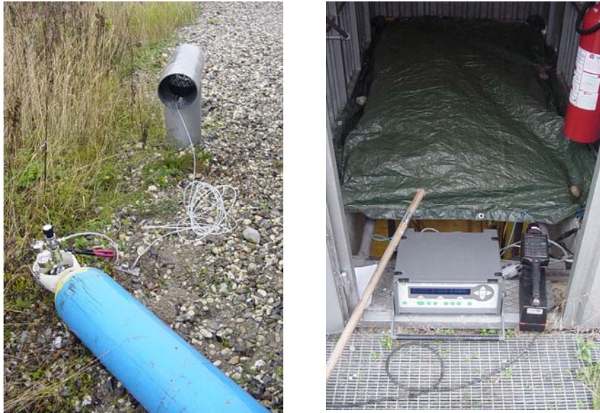
Figure 5.3. Tracer release measurement of methane emission from a leachate pumping station.
