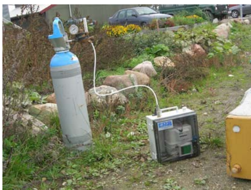
Figure 8.2a. N 2 O tracer release unit, including gas bottle, two-stage regulator and volume integrator.
