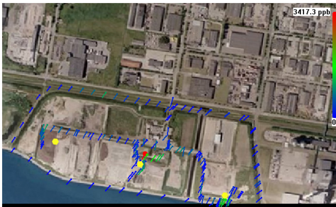
Figure 8.3. Leak search of methane at the AV Miljø landfill area. Color scale and dot size indicate concentration of methane in ppb, sampled 2 m above ground. The scale is linear from 0 to 3417 ppb. The colored lines are pointing up in the wind, and thus indicate potential leak source area. The yellow hexagons indicate positions for the three tracer sources used in the emission quantification.
