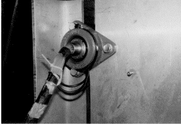
Figure 2-6 The pneumatic plastic tubes exit from the suspension axis of the airfoil section.
