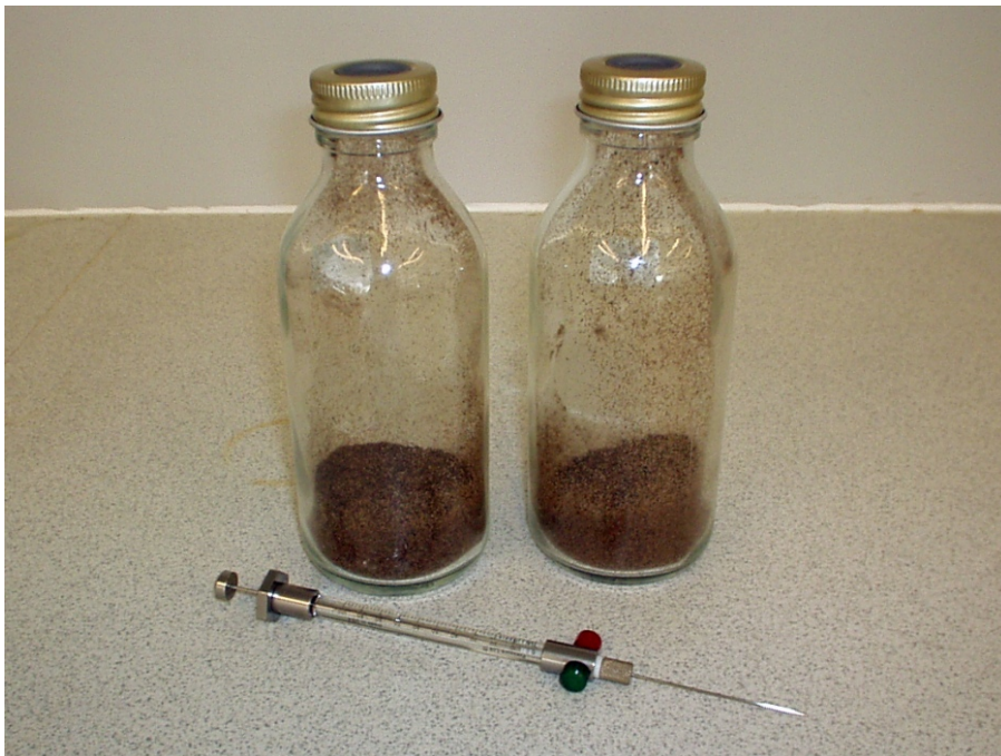
Anaerobic batch experiments with soil. Gas samples for GC-analysis are taken using the shown syringe (gas tight with pressure lock).
