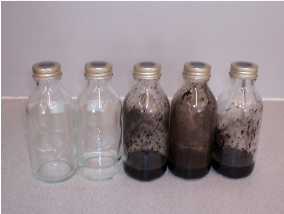
Anaerobic batch experiments with organic waste. The two bottles to the left function as control experiments.
