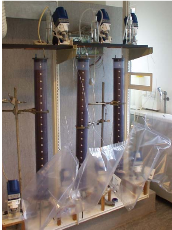
Soil columns equipped with gas sampling port and permeated with artificial landfill gas
