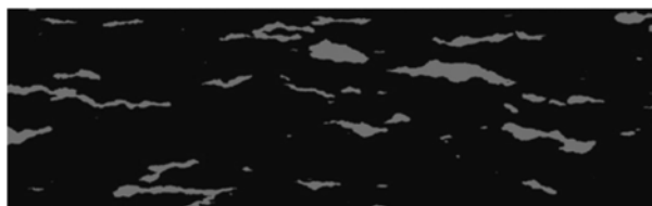
Figure 2: Mapped cross-section indicating the clayey matrix (black) and the sand lenses (grey). The lower two pictures show simulation results with a sequential indicator (SIS) and a multiple-point (MPS) algorithm.
