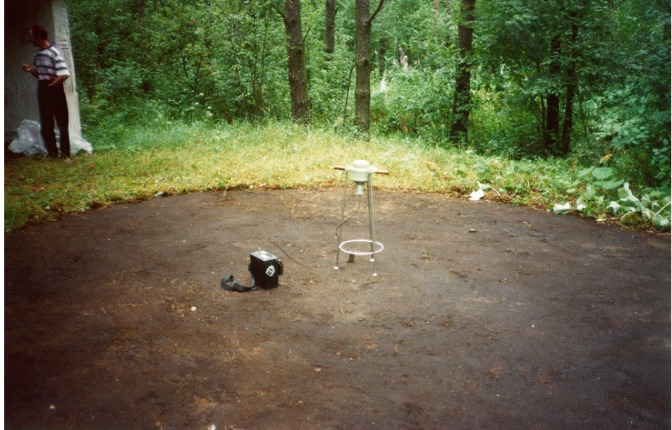
Plate 5.1. The CORAD device measuring the contamination of the asphalted area after removal of the organic cover. The picture shows that the photo-multiplier of the NaI crystal based system is facing down. This is the only opening in the lead collimator surrounding the crystal. The box with the electronics for data collection and treatment is seen to the left in the picture. The measurements are made at a height of 1 m above ground level.
