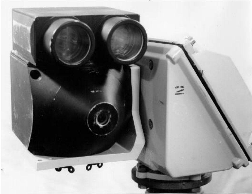
Figure 2.1 The measuring head of the Gamma locator mounted on a pan-and-tilt unit (to the left). On top of the collimator the laser distance device can be seen.
