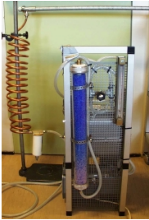
Figure 3.2 Complete mount for total dust measurements. On the left the cooling circuit with a water separator underneath. In the centre a drying column.
