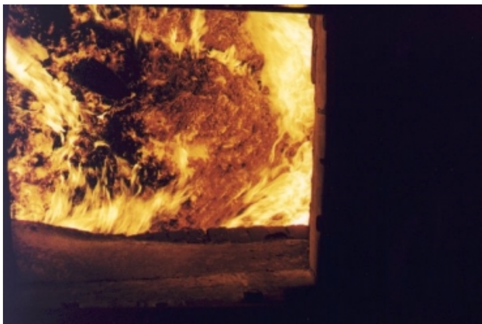
Figure 1.2 Burning wood chips on the grate.
