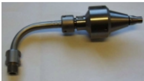
Figure 3.3 Measuring head/filter holder for total dust measurements. The filter holder uses 5 cm Ø quartz fibre filters. The sampling aperture can be adjusted by exchanging the front end of the filter house
