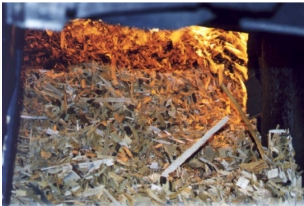
Figure 1.1 Wood chips on the grate right after fuel addition.
