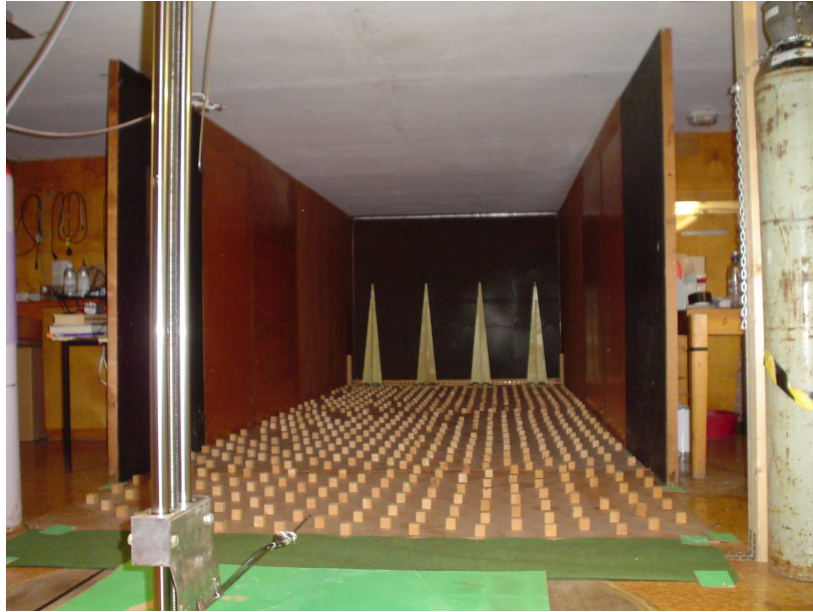
Fig. 1.4.1. View of the roughness configuration in BLWT of NUI, Galway
