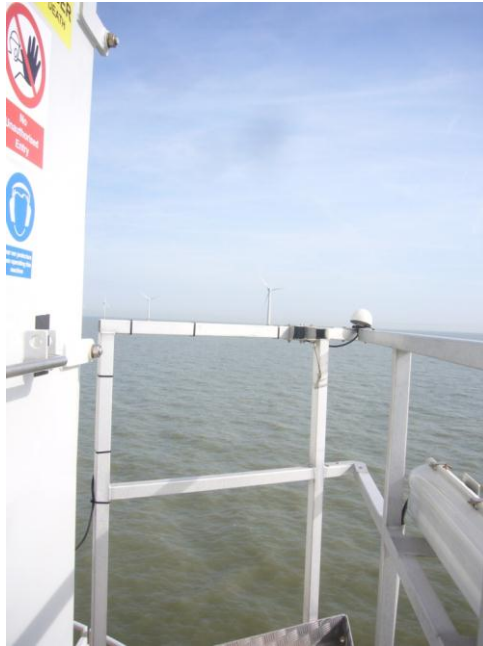
Fig. 3 GPS antenna installed on the service stairs of a wind turbine in Gunfleet Sands.
