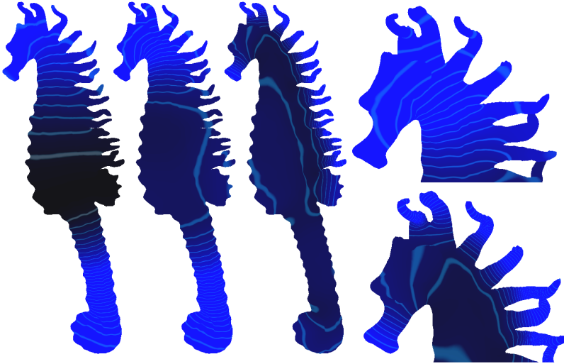
Figure 5.3: ADF evaluated with t equal to respectively 2, \frac{1}{2} , and \frac{1}{32} (left to right). In the magnified images t is \frac{1}{2} (top) and \frac{1}{32} (bottom). The lines show the isocontours of the function; brighter color indicates bigger value of the ADF.
