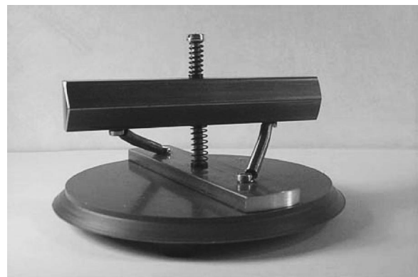
FIG. 1. The experimental setup that consists of two (upper and lower) helically rotating coupled plates. The supporting bottom plate creates friction for the lower plate. A driving oscillating or fluctuating force is applied to the upper plate, e.g., by hitting it slightly from various directions. Colored noise was created by the sound from a fog horn, acting on a horizontal membrane glued on top of the upper plate. In all cases of forcing vertically (from above or below), the helical system was observed to rotate only clockwise when viewed from above.
