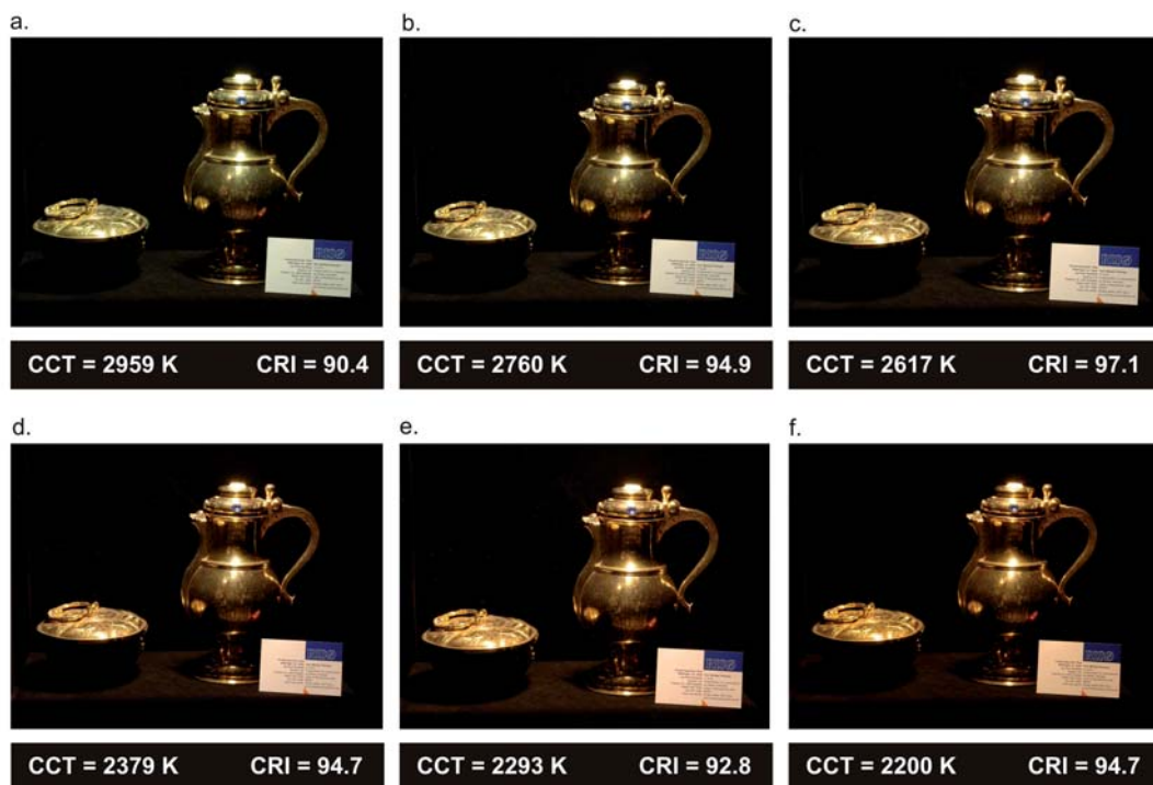
Fig. 5.2. Photos of gold samples under LED illumination at different correlated color temperatures. a. Illumination of gold samples using a commercial Lumileds LED. b–f. Illumination of gold samples when the correlated color temperature of the new LED light source is reduced from 2760 K to achieve the desired 2200 K (F). CRI: color-rendering index.
