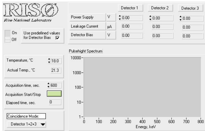
Figure 3.2. The LabView© front plate is designed to display puls-height distributions for any choice of coincidence mode. In addition a number of control parameters are displayed.
