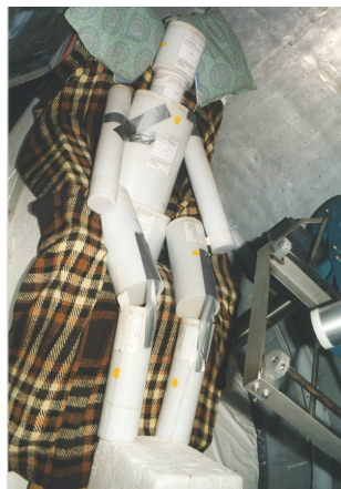
Figure 5.2. The BOMAB phantom in the chair at Risø's whole body counter; the germanium detector is not in the measuring position
