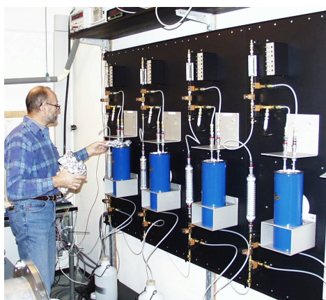
Figure 2.8. Seawater radon extraction systems.
