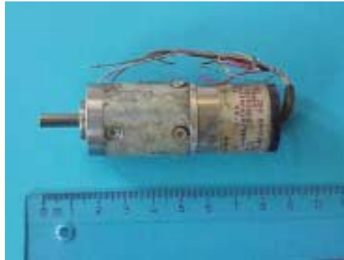
Figure 5.1. Step motor used in a triple axis spectrometer at Reactor DR 3.
