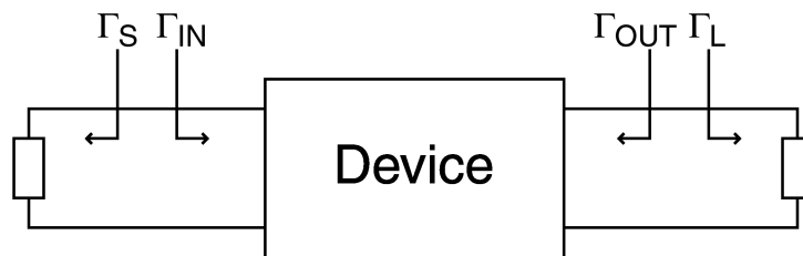
Figure 3.2 Definition of impedances used for matching a two-port.
