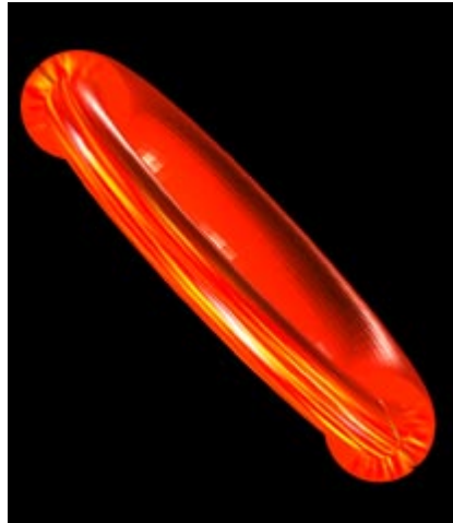
Figure 39. Colour plot of the density calculated with the full toroidal code. The structures visible tend to align to the magnetic field, winding around the torus with a winding number of q = 2.34 .
