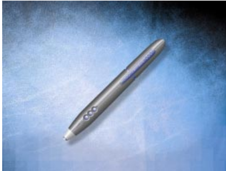
Figure 33. FreePen : The optical system for tracking the rotation of the ball is placed below the three buttons at a distance of 17 mm. The optical head including laser and detectors has a diameter of 6.8 mm.
