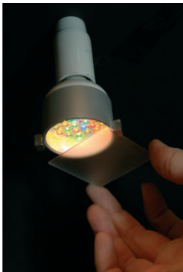
Figure 13: Early demonstration from the Danish LED project: A micro-structured optical plate mixes light from coloured LEDs to form “white” light of high quality with low electrical power consumption.
