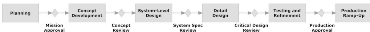
Figure 6: The generic product development process (also called the stage gate model). Source: Ulrich & Eppinger (2008)
