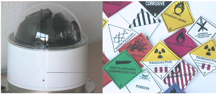
Figure 18. A controllable camera is used to locate and classify danger labels on containers.
