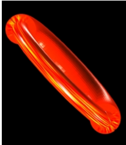
Figure 8. Colour plot of the density calculated with the full toroidal code. The structures visible tend to align to the magnetic field, winding around the torus with a winding number of q = 2.34 .
