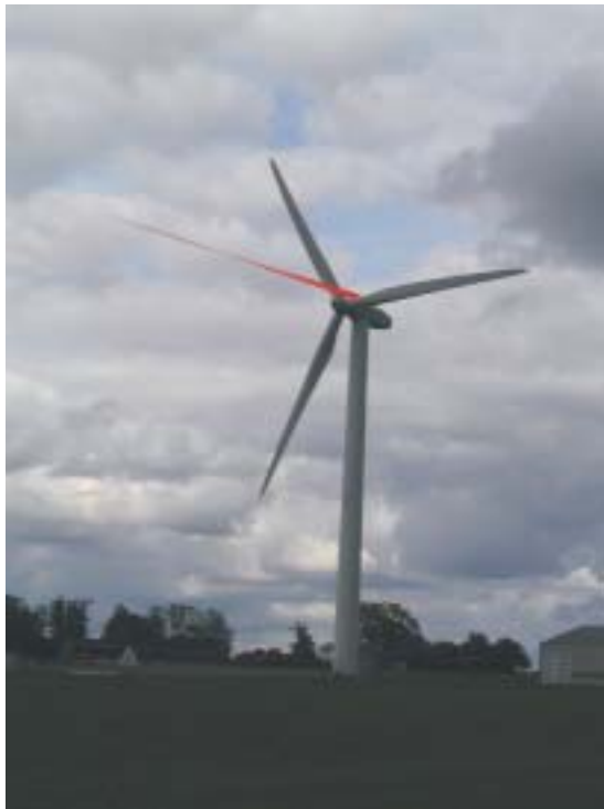
Figure 35. An artistic impression of the otherwise invisible laser beam, emitted from the laser anemometer.
