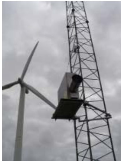
Figure 37. The final demonstration instrument mounted on a test platform on a mast in front of the large wind turbine at the Risø test site. The anemometer measures the wind velocity coming from Roskilde Fjord.
