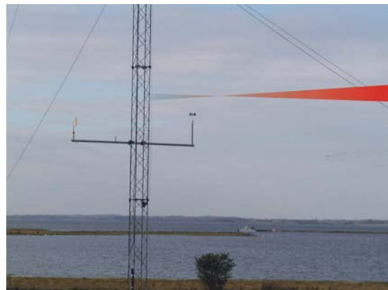
Figure 44. The laser beam was focused nearby a conventional cup anemometer for comparison during measurements.
