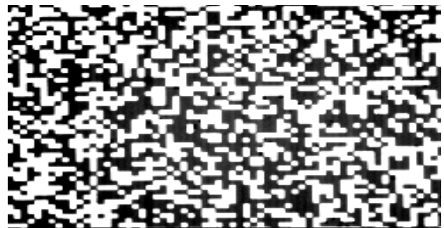
Figure 18. 2D representation of a section of a computer-generated binary holographic diffuser.
