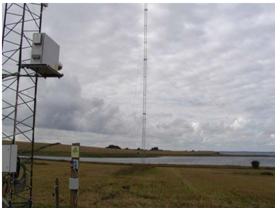
Figure 43. The final demonstration instrument mounted on a test platform on a mast in front of the large wind turbine on the Risø test site. The anemometer measures the wind velocity coming from Roskilde Fjord. The whole laser instrument is controlled from and transmits the measurements through the Internet.
