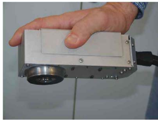
Figure 26. The mobile OCT system in the clinic and the compact handheld probe.
