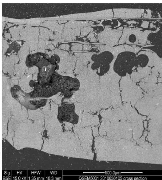
Figure 5.4 Reference catalyst plate exposed for 850 hours with potassium chloride. Surface potassium concentration (top) 6.3 wt%; potassium concentration along the catalyst plate cross section (bottom).
