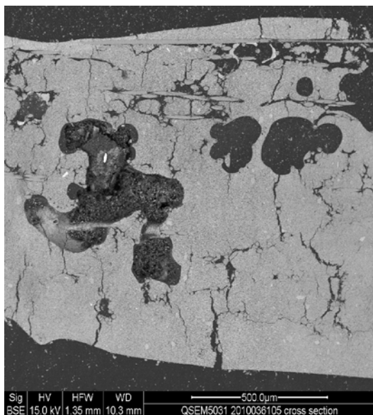
Figure 7.3 Reference catalyst plate exposed for 850 hours with potassium chloride. Surface potassium concentration (top) 6.2 wt%; potassium concentration along the catalyst plate cross section (bottom).
