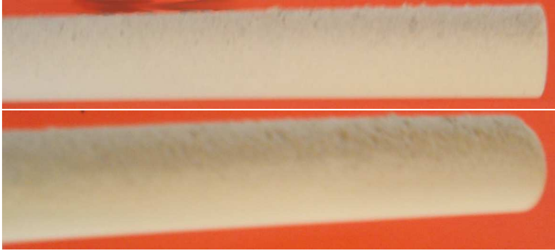
Figure 3.13: View of deposits from the side. The deposit probe has a diameter of 16 mm and the thickness of the upstream deposits is about 1 mm. Top: coal/air combustion; Bottom: coal/oxyfuel combustion. The upstream part of the probe faces upwards in the picture. Colour differences are a consequence of the picture recording.
