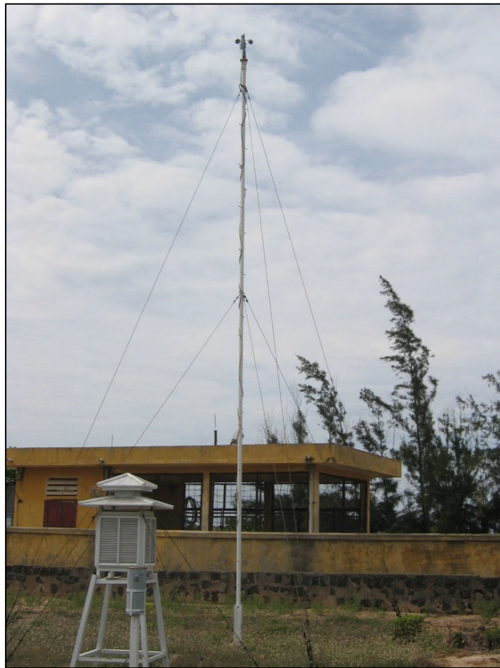
Figure 28: The 12 m met-mast at the Ly Son Met-Station that may provide long term wind reference. (Photo: RISO 2006)
