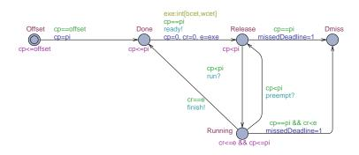
Figure 5.7: Basic timed-automata skeleton for tasks
