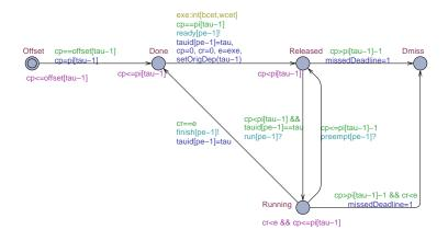
Figure 5.9: Timed-automata skeleton for tasks with platform communication
