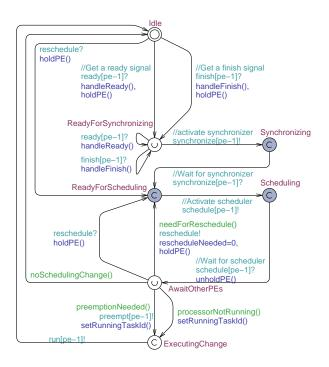
Figure 5.4: Full timed-automaton template for controllers
