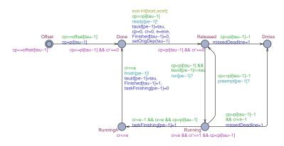
Figure 5.11: Task model using stop-watch automata
