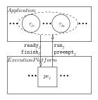
Figure 5.2: Communication between execution platform and application
