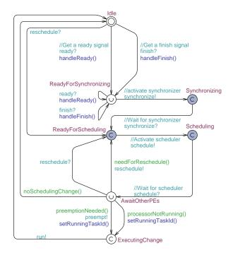
Figure 5.3: Basic timed-automata template for controllers
