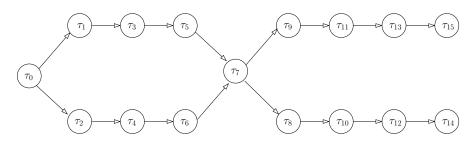
Figure 2.2: Task graph of an MP3 decoder
