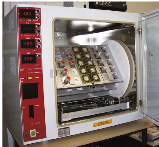
Figure 4.8: Tilting table for the integration of the roller-tube technique with a MEA. A drummer inside the incubator space keeps rolling to switch the culture in a submerged state in medium and breathing in contact with air [82]
