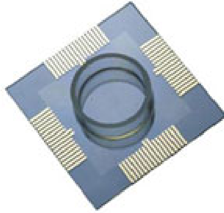
Figure 4.9: A commercial MEA chip with attached ring for interface culture. The area inside the ring will be the site for the culture of the brain slice by the interface method (image taken from [83])
