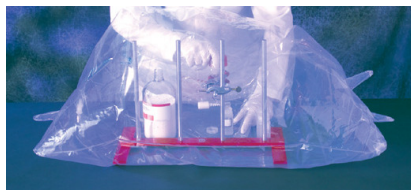
Fig. 2.4.3 Polyethylene bag with integrated gloves. The snippets at the sides were used for flushing with nitrogen and inlets for electrical cords.
