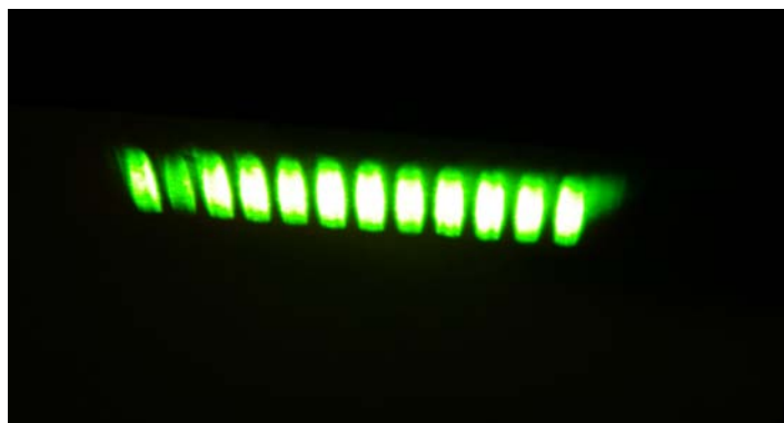
Fig. 3.3. Near field photograph of the tapered diode laser bar at I= 10A .
