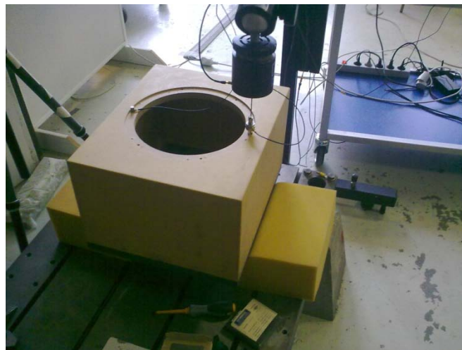
Figure A-2. Loudspeaker cabinet placed on soft foam.
