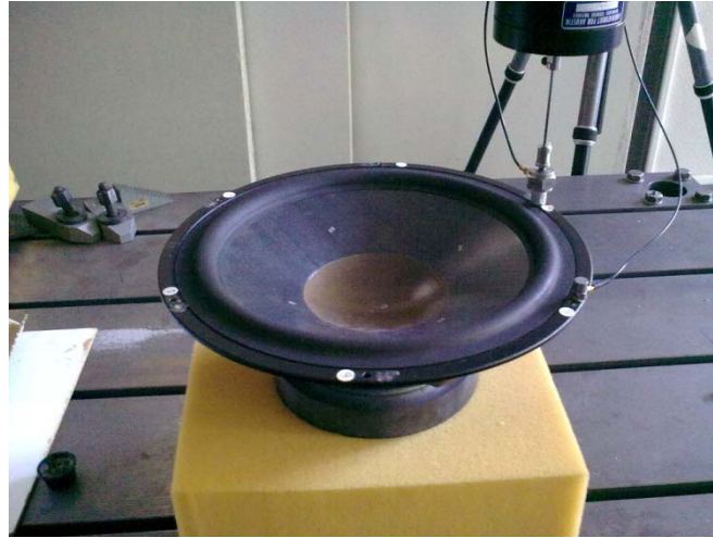
Figure A-1. The 10 inch loudspeaker unit placed on soft foam.
