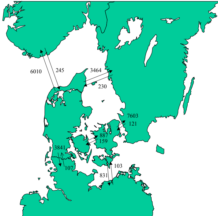
Figure 6.3. Exchange of energy (GWh/year). CO_2 tax: 0 DKK/tonne.
