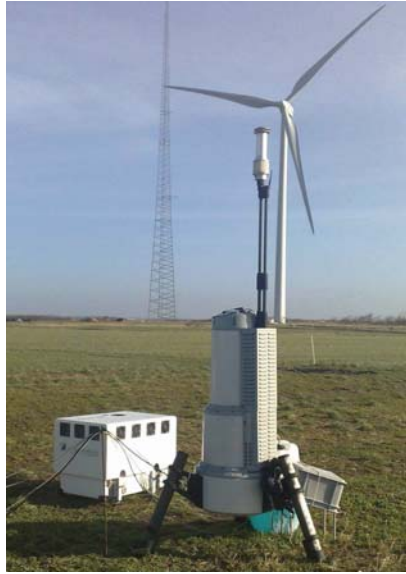
Figure 6.1: Picture of a Windcube lidar (on the left) and a ZephIR lidar (on the right)
