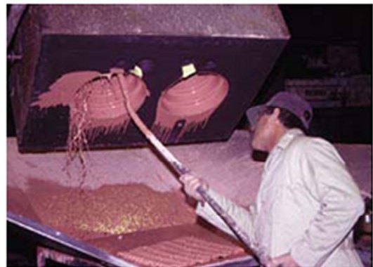
Figure 6. Flow coating method, it is seen that the mould is inclined at an angle.
