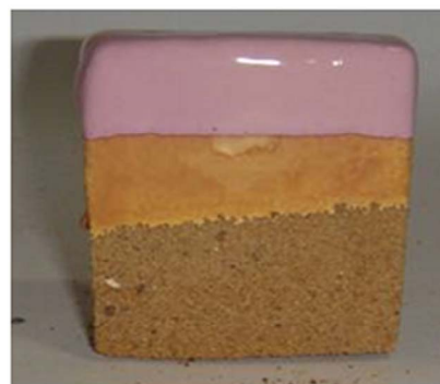
Figure 7. Colour changing Zircon Foundry Coatings changes colour from Yellow to Pink, Pink to Yellow on drying or ignition. Available both in Water and Solvent based [43].
