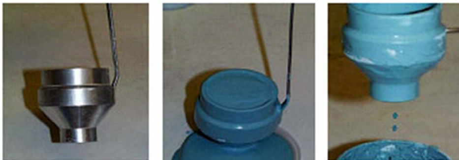
Figure 8. Measurement of viscosity with a flow cup [45].
