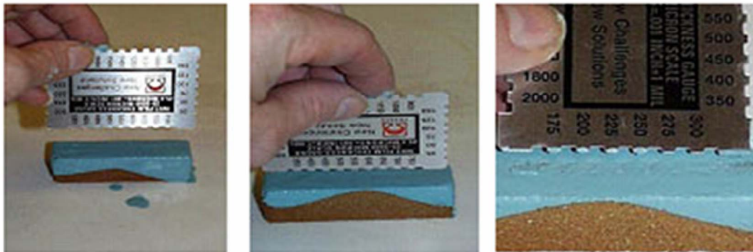
Figure 10. Measuring the wet thick layer of a coating [45].
