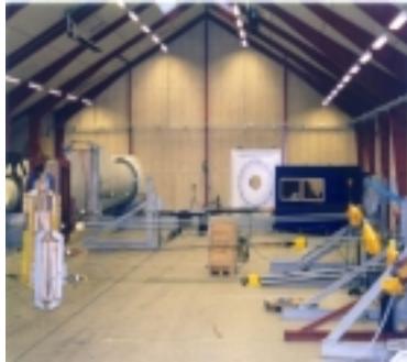
Figure 9. Flap-wise static test of a wind turbine blade at Risø Sparkær Centre.
