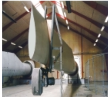
Figure 11. Chord-wise fatigue test of a wind turbine blade at Risø Sparkær Centre.
