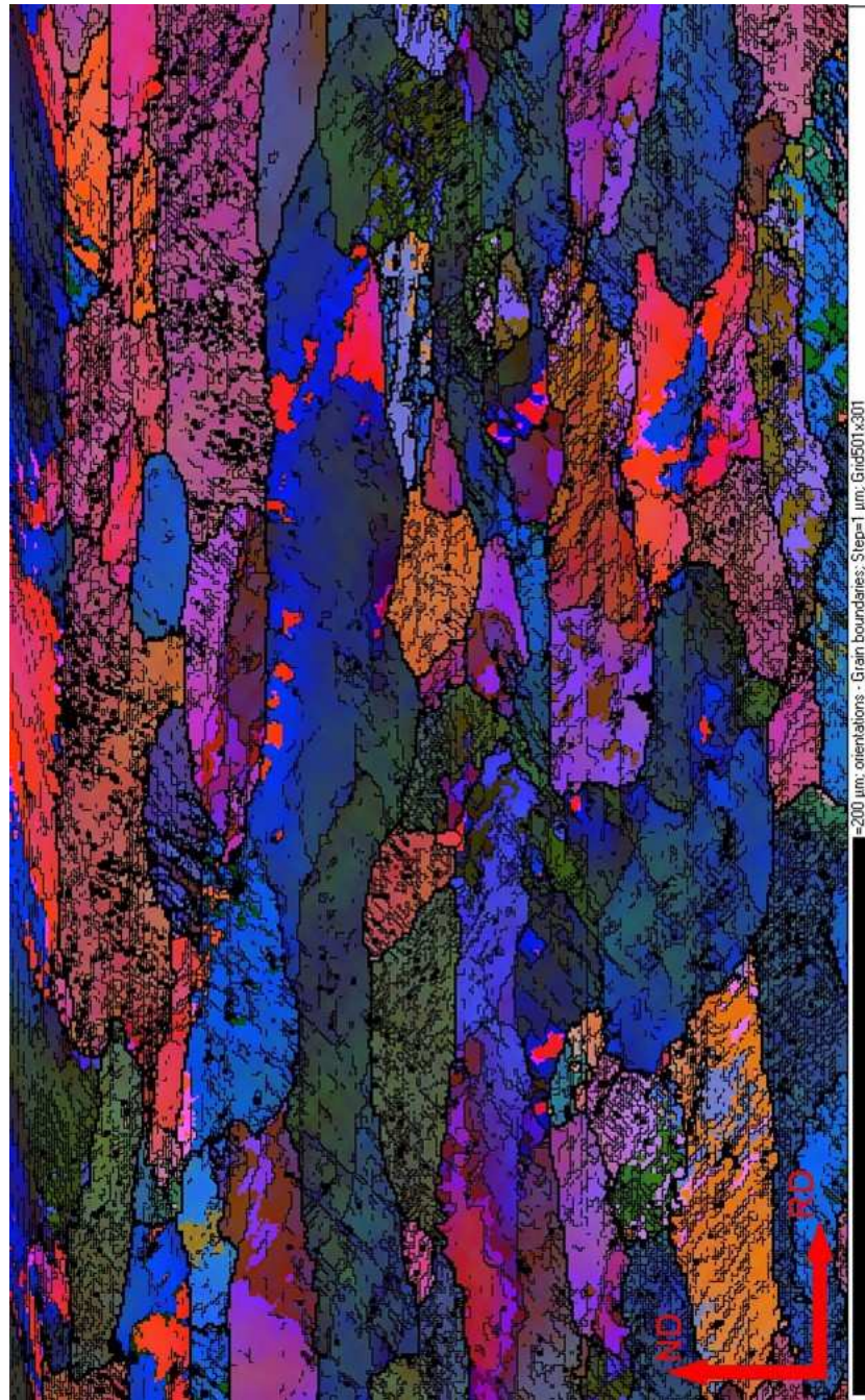
Figure 5.4: EBSD orientation map of an sample annealed at 231°C for 3 hours. Misorientations larger than 3° are marked with thin black lines and misorientations larger than 15° are marked with thick black lines.
