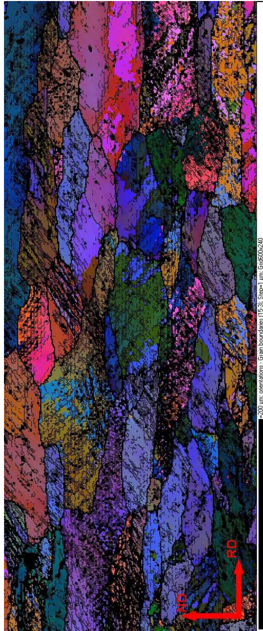
Figure 5.3: EBSD orientation map of an as-deformed sample. Misorientations larger than 3^\circ are marked with thin black lines and misorientations larger than 15^\circ are marked with thick black lines.
