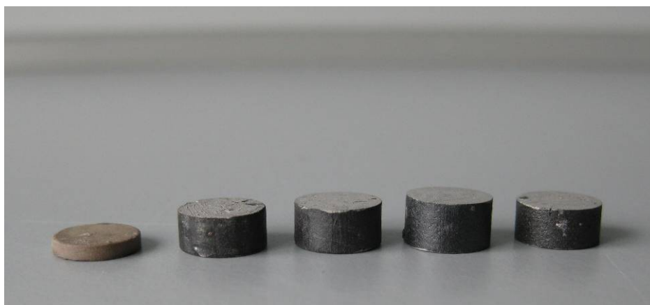
Figure 14 NiSCY pellets, with 0, 0.5, 1, 2 and 4 % Ni
