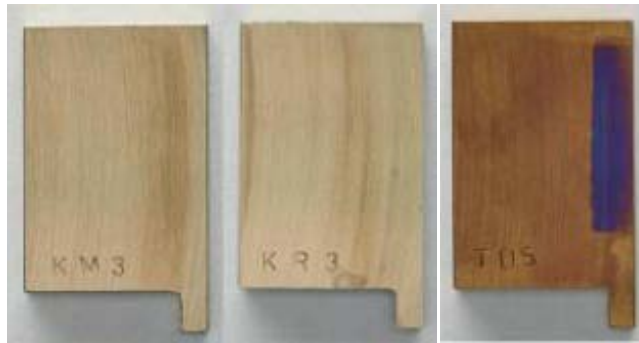
Fig. 2: Example images of coupons (from left to right, 1.4006, 1.4313, 1.1018) after 600 hours at 170 °C in continuous CO 2 stream at atmospheric pressure, elevated amounts of impurities.
