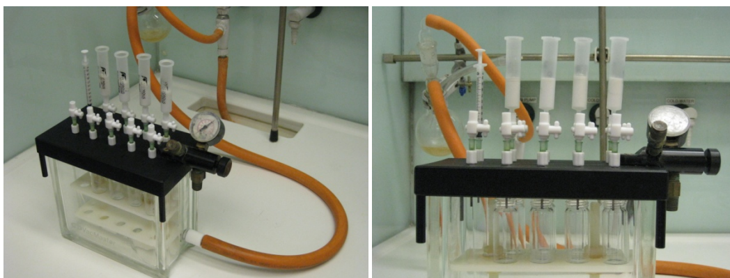
Figure 61. Pictures of 10 port SPE vacuum manifold with F-SPE cartridges.
